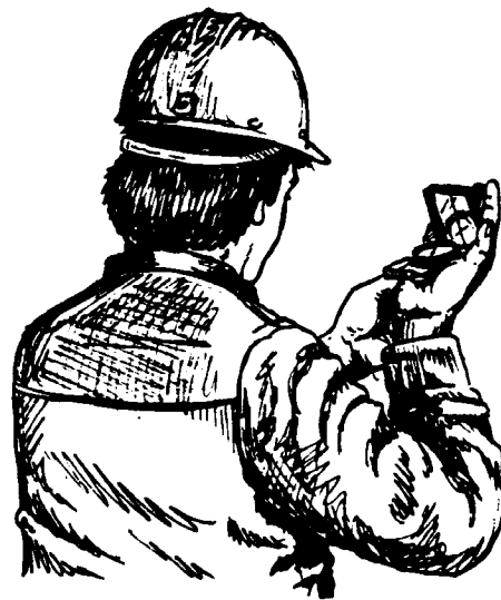
Figure 4-26. Taking an azimuth with a Silva compass.
