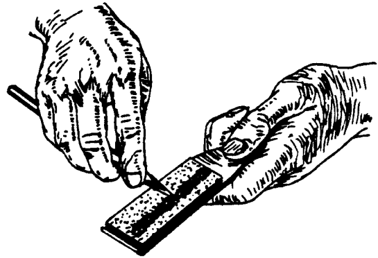
Figure 10-8. Use of sandpaper block to sharpen pencil for drafting maps.
