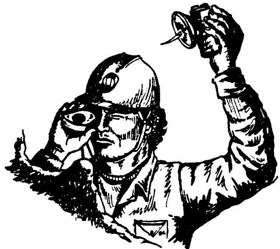
Figure 4-21. Using a lamp to illuminate the Suunto compass while taking an azimuth reading.
